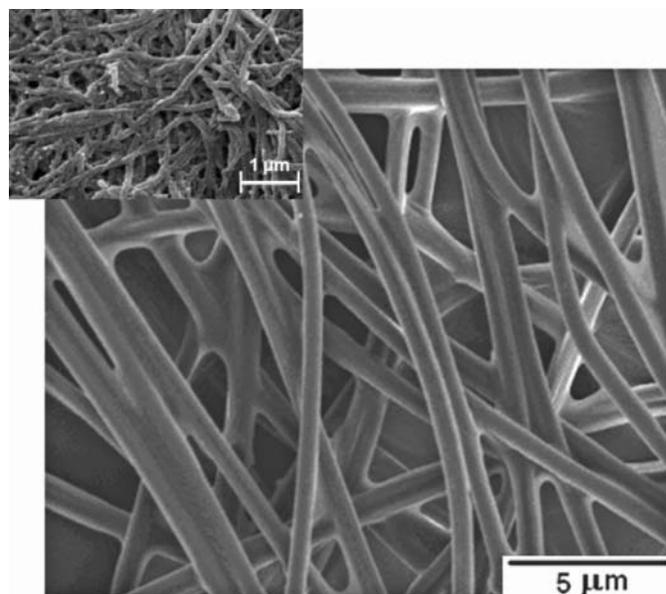
**Fig. 2.** SEM micrograph of the HPLy-PANINTs electrospun fibers at a PANINTs concentration of 1.5% w/w. The inset in the upper left shows the micrograph of the PANI nanotubes used for HPLys-PANINTs nanofibers fabrication.
