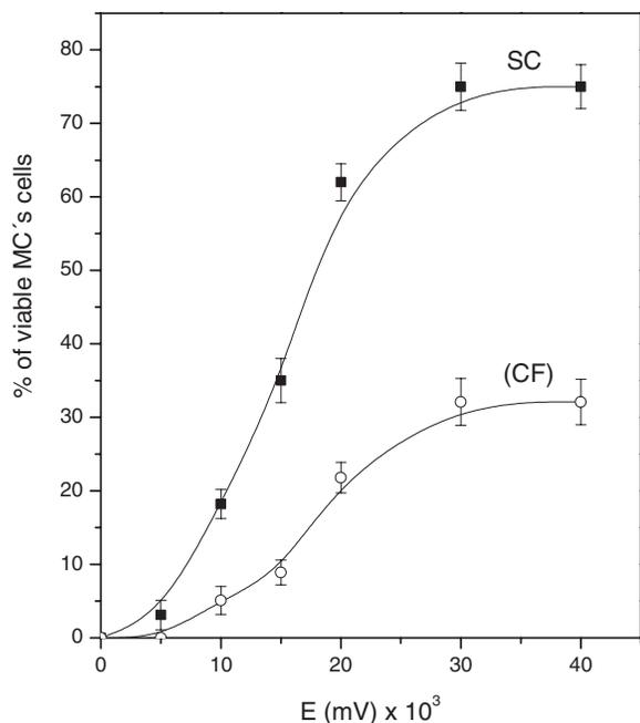
**Fig. 5.** Effects of electrostimulation on cell growth after 72 h. SC (■) and CF (○) are fibrous scaffold and cast HPLys-PANINTs films, respectively. (PANINTs concentration in the nanofiber was 1.5% w/w).
