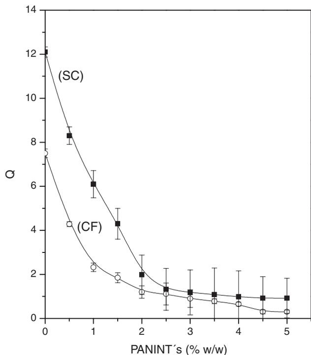
**Fig. 3.** Swelling behavior of the HPLys-PANINTs electrospun fibers. SC (■) and CF (○) are fibrous scaffold and casting HPLys-PANINTs, respectively.
