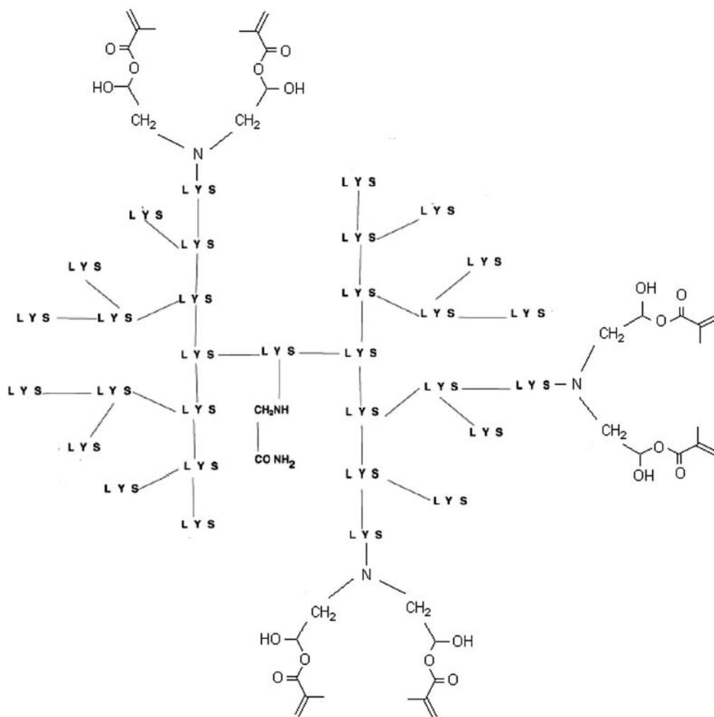
**Fig. 1.** Illustrative structure of epoxidized HPLys after reaction with GMA.
